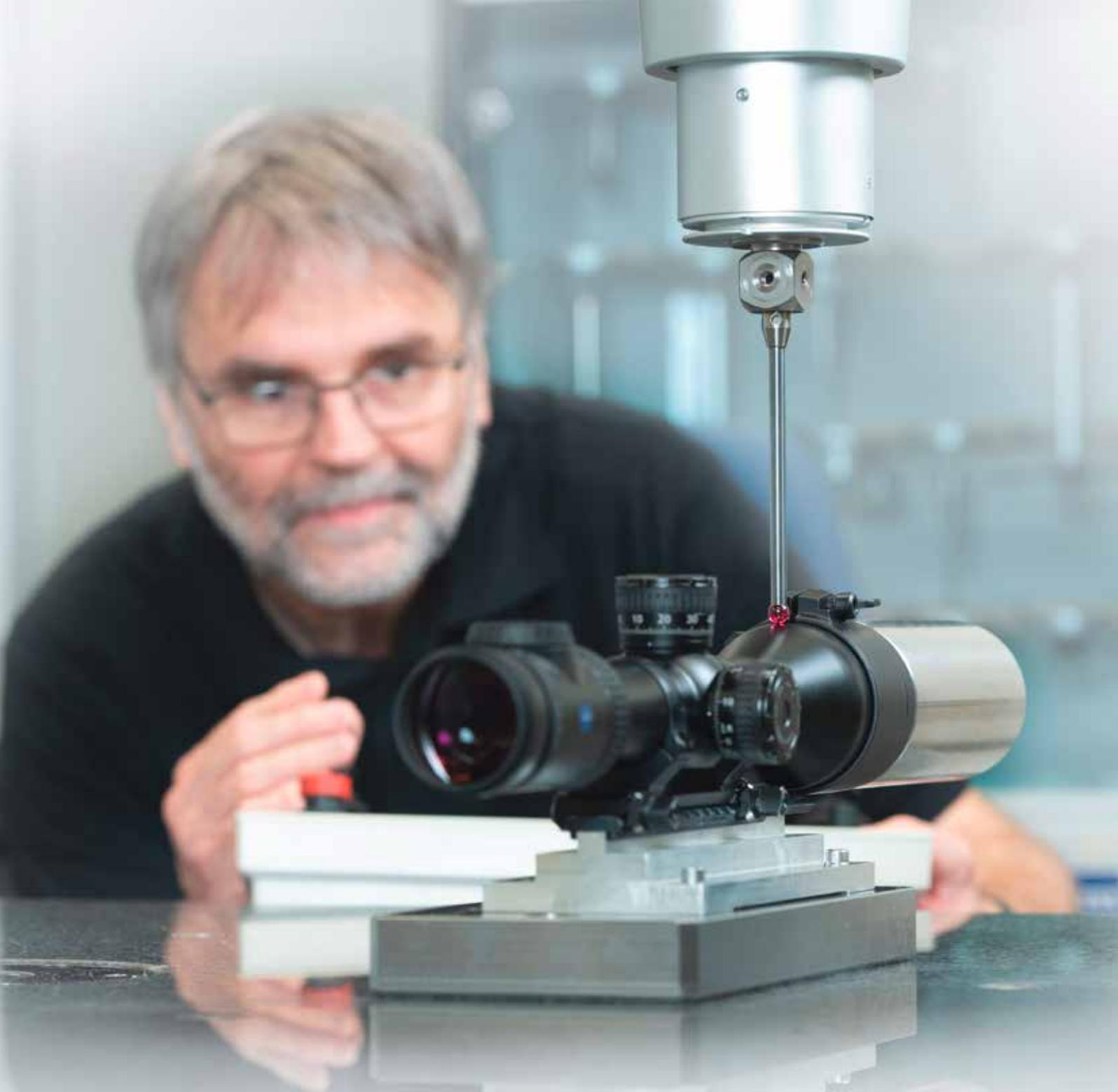
Since riflescopes are exposed to extreme recoil and vibration forces during firing, the ZEISS laboratory not only carried out mechanical tests on the possible deflection and rigidity of the riflescopes, but also placed considerable emphasis on the deviation from the target line by using attachments and adapters.
