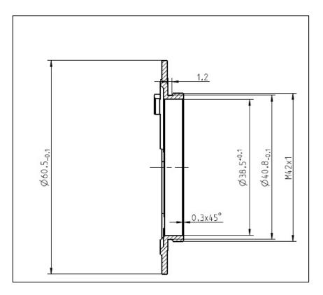
The diameter of the camera/lens adapter must not exceed 60 mm at the interface to the lens!
